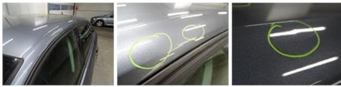
Roof pillar R, Hail damage, PDR - Hail
