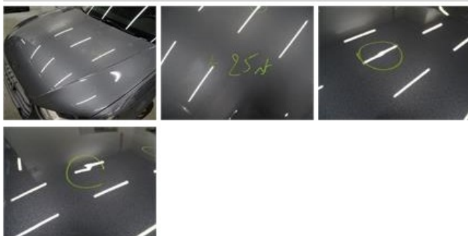
Roof, Hail damage, LI - Repair and paint (complete)
