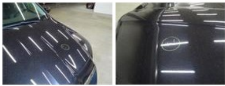
Roof, Dent(s), PDR - Paintless dent repair
