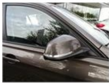
Rearview mirror housing R, Scratch(es), Smart repair
