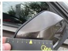
Rearview mirror housing R, Scratch(es), Smart repair
