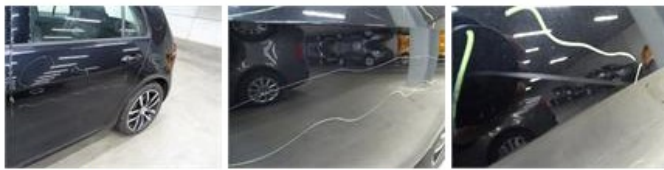
Bonnet, Chemical pollution, LI - Repair and paint (complete)
