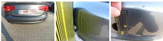
Door panel F L, Tear, Smart repair
