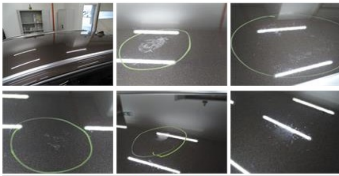
Door F R, Bad repair, LI - Repair and paint (complete)
