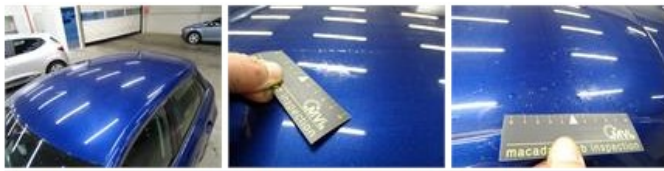
Wing R L, Chemical polution, LI - Repair and paint (complete)
