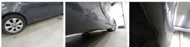
Protection plate M, Deformed / Strained, E - Replace
