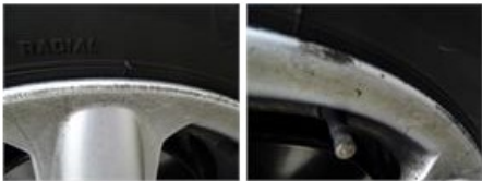
Tyre R R, Deformed / Strained, E - Replace
