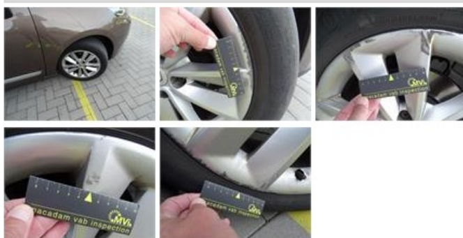
Tyre F R, Worn, E - Replace
