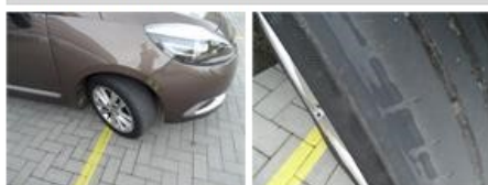
Wheel bolt cover F L, Damaged, E - Replace
