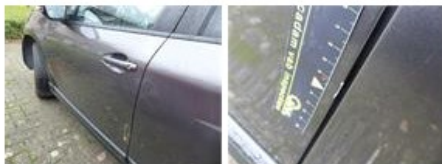
Wing F L, Dent(s), It - Spot repair
