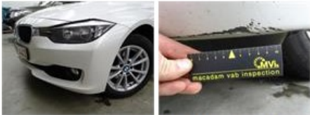
Bumper R, Deformed / Strained, LI - Repair and paint (complete)
