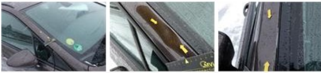
Rearview mirror basis L, Broken, E - Replace
