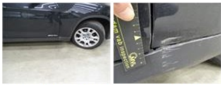
Sill outer R, Dent(s) and scratch(es), It - Spot repair
