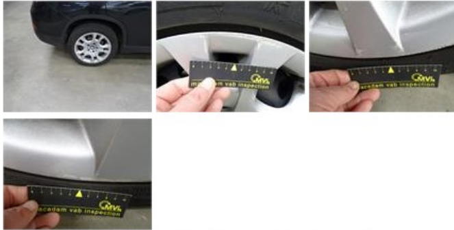
Wing R R, Dent(s) and scratch(es), LI - Repair and paint (complete)
