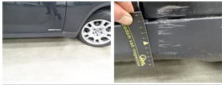
Wheel cover R R, Scratch(es), E - Replace
