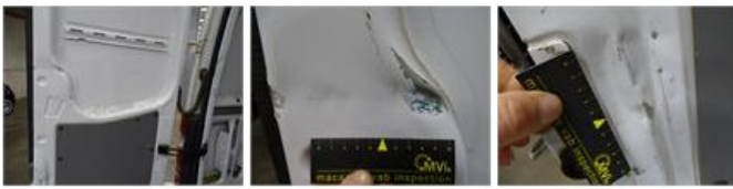
Spare wheel compartment lining R R, Dent(s), Smart repair
