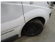
Wheel cover F R, Missing, E - Replace
