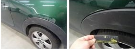
Wheel arch cover R L, Scratch(es), E - Replace
