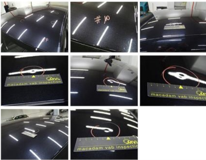
Roof pillar L, Hail damage, PDR - Hail 0,00
