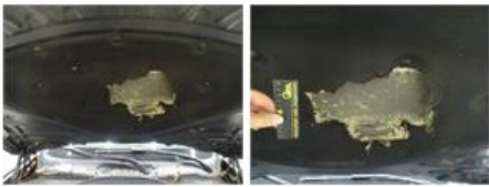
Engine protective plate, Deformed / Strained, E - Replace
