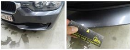
Engine protective plate, Deformed / Strained, E - Replace
