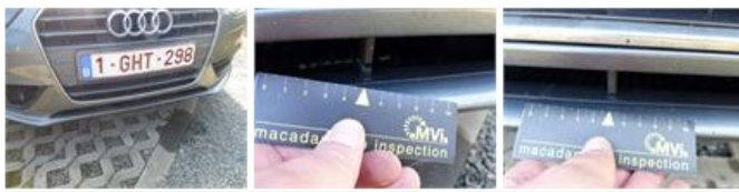
Bumper F, Deformed / Strained, Le - Replace and paint
