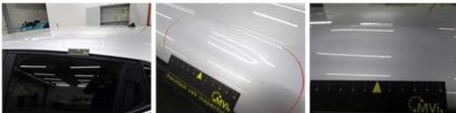
Wing R R, Scratch(es), LI - Repair and paint (complete) 246,56
