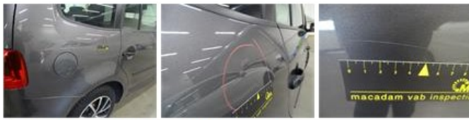
Wing F L, Dent(s), LI - Repair and paint (complete)
