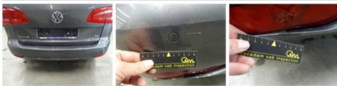
Bumper R, Broken, Le - Replace and paint
