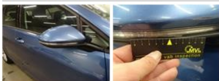
Wing R R, Dent(s), LI - Repair and paint (complete)
