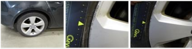
Alloy rim F R, Scratch(es), LI - Repair and paint (complete)
