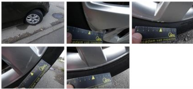
Alloy rim F L, Scratch(es), LI - Repair and paint (complete)
