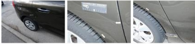
Door R R, Scratch(es), LI - Repair and paint (complete)
