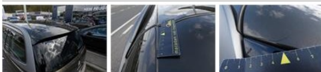
Tailgate, Crack, Le - Replace and paint
