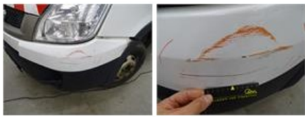
Wing R L, Dent(s) and scratch(es), LI - Repair and paint (complete)
