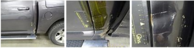
Door R R, Dent(s) and scratch(es), Le - Replace and paint
