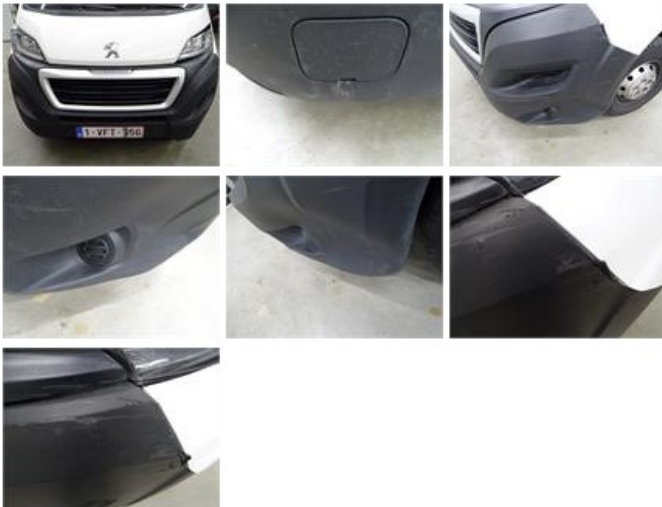
Wing F L, Bad repair, Le - Replace and paint 427,51
