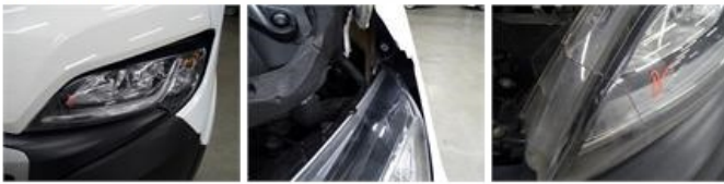
Bumper F, Deformed / Strained, E - Replace 398,40
