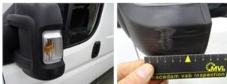
Rearview mirror R complete, Broken, E - Replace
