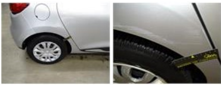
Wheel cover F R, Broken, E - Replace
