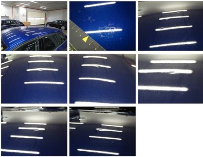
Bonnet, Chemical pollution, LI - Repair and paint (complete) 0,00
