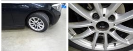
Wheel hub cap R L, Missing, E - Replace
