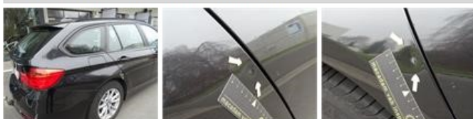
Door F L, Deformed / Strained, LI - Repair and paint (complete)
