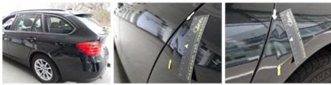
Roof rail L, Deformed / Strained, E - Replace
