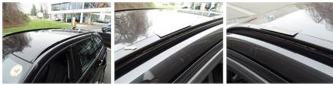
Roof pillar R, Scratch(es), LI - Repair and paint (complete)
