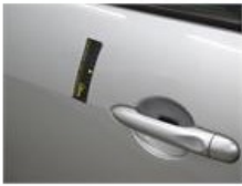
Door R L, Dent(s), LI - Repair and paint (complete)
