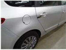
Door R L, Dent(s), LI - Repair and paint (complete)
