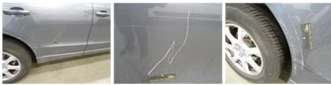
Door moulding Lower R R, Scratch(es), Smart repair
