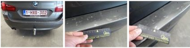
Bumper grille F R, Missing, E - Replace
