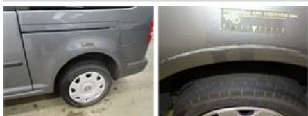
Sill outer R, Dent(s) and scratch(es), LI - Repair and paint (complete)
