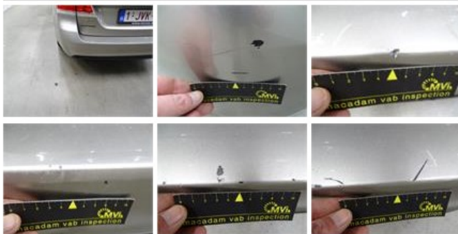
Roof pillar R, Dent(s), Acceptable
