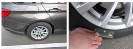
Door panel F L, Scratch(es), Acceptable
