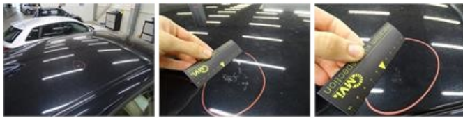
Roof pillar L, Chemical polution, LI - Repair and paint (complete)
