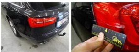
Rearlight L, Crack, E - Replace
