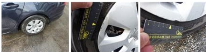
Bumper F, Scratch(es), LI - Repair and paint (complete)
