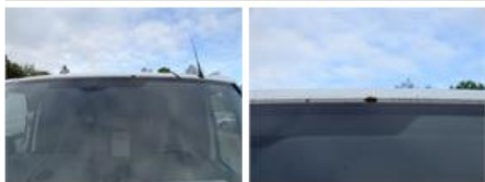
Aerial, Damaged, E - Replace
