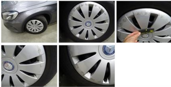
Wheel cover F R, Scratch(es), Acceptable
