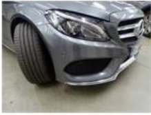
Bumper moulding F R, Scratch(es), E - Replace
