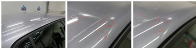
Roof pillar R, Hail damage, PDR - Hail
