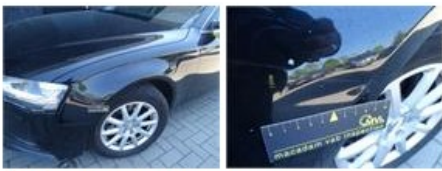
Bumper F, Dent(s), LI - Repair and paint (complete)
