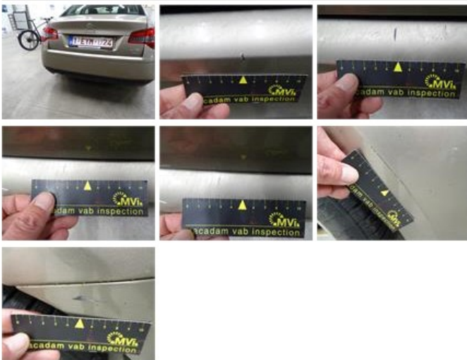
Sill outer L, Dent(s), It - Spot repair
