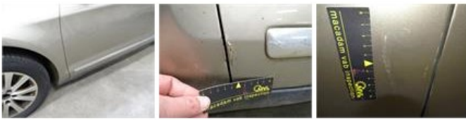
Wing F L, Scratch(es), LI - Repair and paint (complete)
