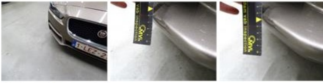
Bumper F, Dent(s), LI - Repair and paint (complete)
