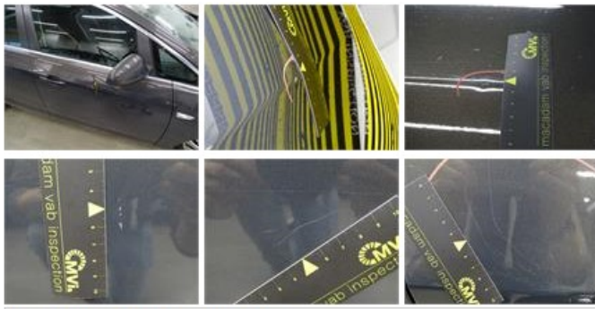
Protection plate M, Tear, E - Replace
