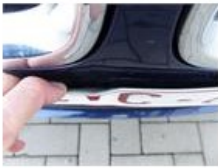
Sill outer R, Dent(s) and scratch(es), LI - Repair and paint (complete)
